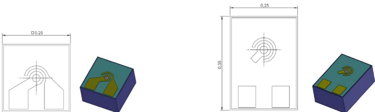
**Figure 2:** VCSEL interface layout. Left: conventional layout, right: configuration for WB and NFC.
