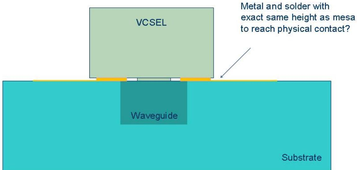
**Figure 1:** Near-field coupling and flip chip
