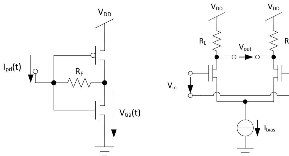
**Figure 10: Schematics of an inverter-based TIA with resistive feedback and differential amplifier.**
