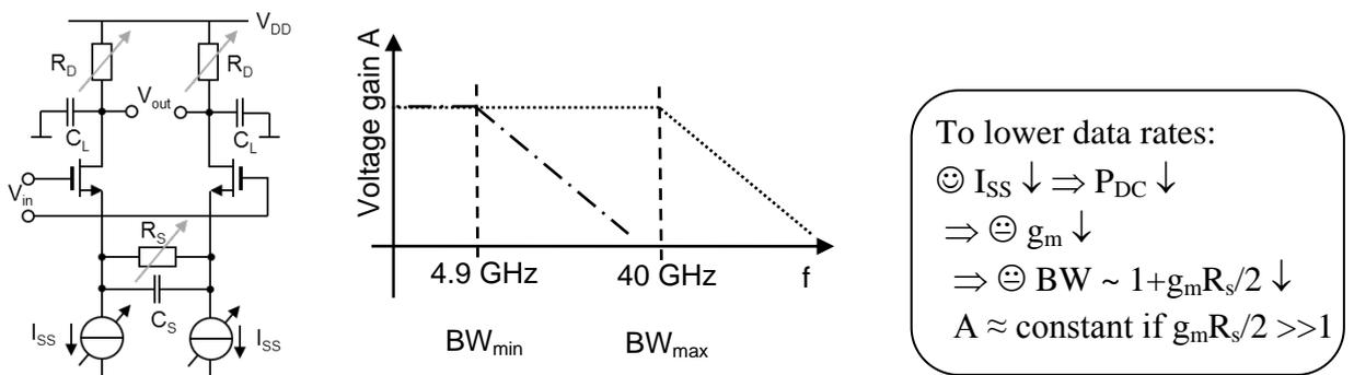
Figure 3: Adaptive tuning of a LA; (left) concept, (middle) frequency response, (right) functional chain.
