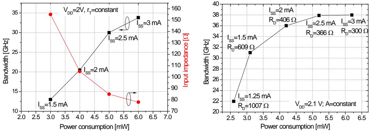
Figure 7: Simulation of adaptive tuning for (left) TIA and (right) LDD.
