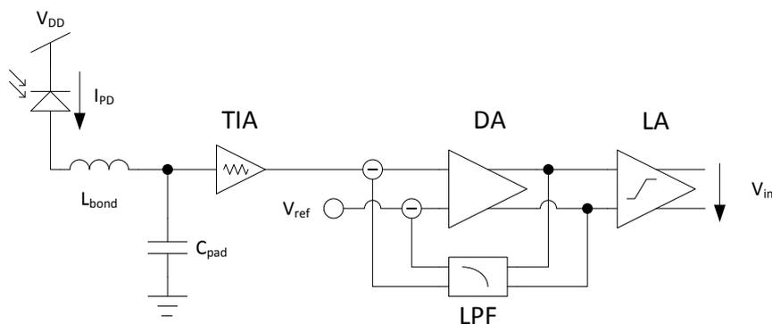
**Figure 9: Optical front-end subsystem.**
