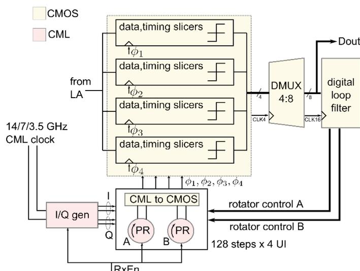
**Figure 13: CDR Block diagram. The bias current of PRs and I/Q generation can be turned off to save power while the link is idle.**
