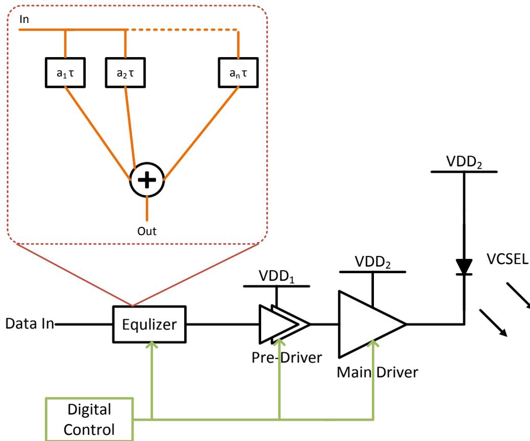
Figure 8: An overview of the transmitter chip.
