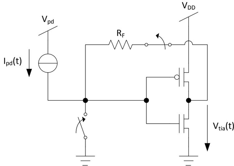
**Figure 11: Inverter Based TIA with on/off adaptivity.**
