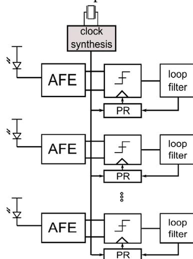
**Figure 12: Embedded clock optical link with reference clock.**
