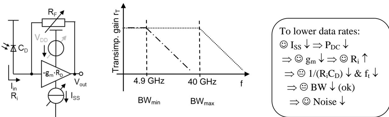
Figure 2: Adaptive tuning of a TIA; (left) concept, (middle) frequency response, (right) functional chain.
