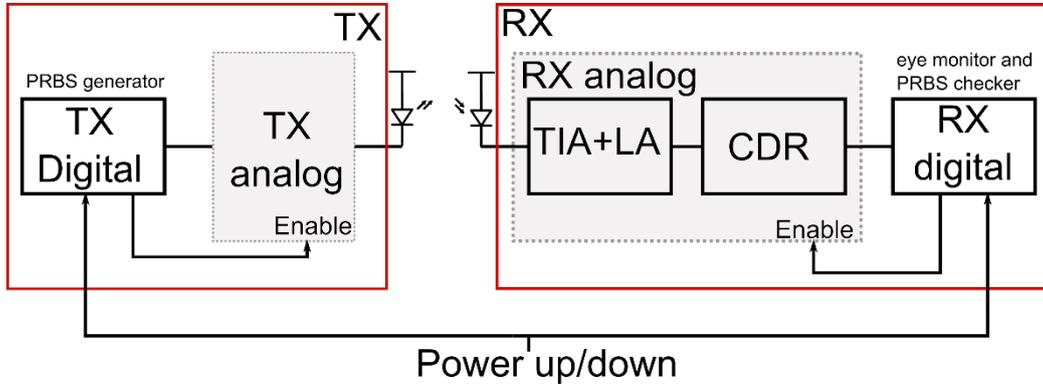
**Figure 1: High level block diagram of adaptive optical link path outlining digitally assisted TX/RX analog macro.**
